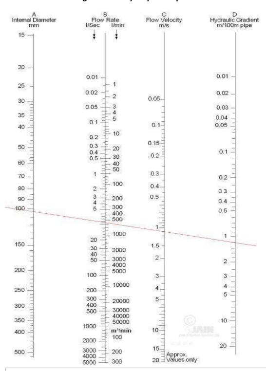
**Example:**Flow 10 lps, Pipe size 110 mm OD (104mm ID), Velocity 1.2 m/s, Hydraulic Gradient 1.2 m/100m.
